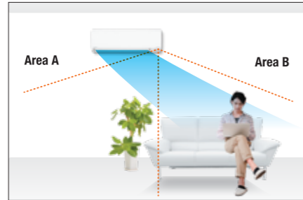
If a person is detected in area B, airflow is directed toward area B.
