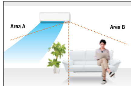
If a person is detected in area B, airflow is directed toward area A.
